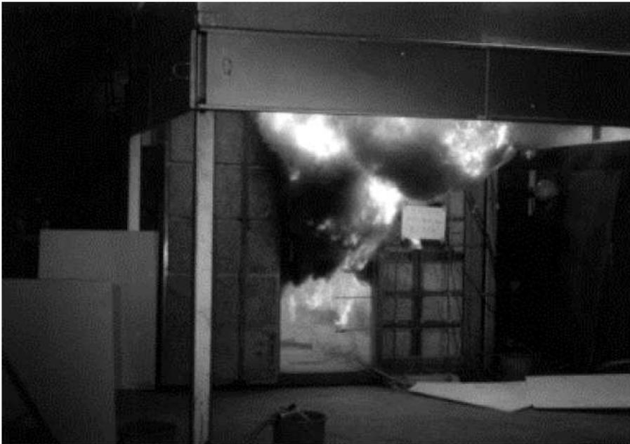
Photo 4.1 Flashover at room corner test ISO 9705
